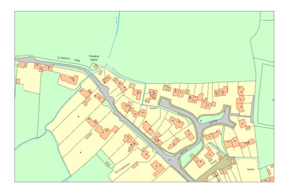
The means of surface water disposal is another matter however and it is intended to discharge excess surface water to an existing open watercourse shown above. The open watercourse is coloured blue and runs from the hammerhead at the western end of Dutts to the Wessex Water pumping station and out across the fields in a larger open watercourse. This receiving watercourse fronts the proposed property and is shown in the photograph below.
